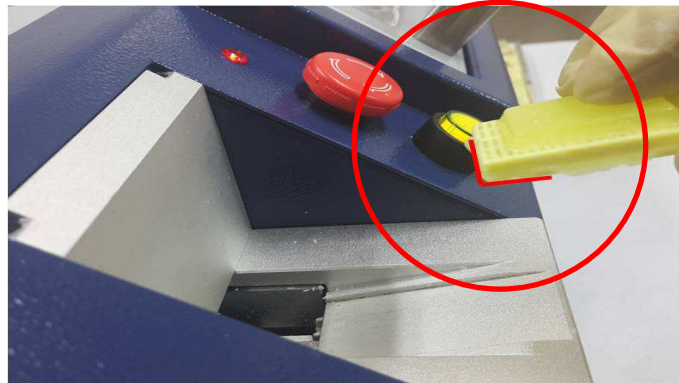
< Wrong way to put the block into the inlet >
